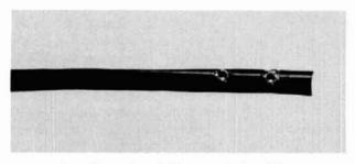
Sample section of a homemade fluted line.
